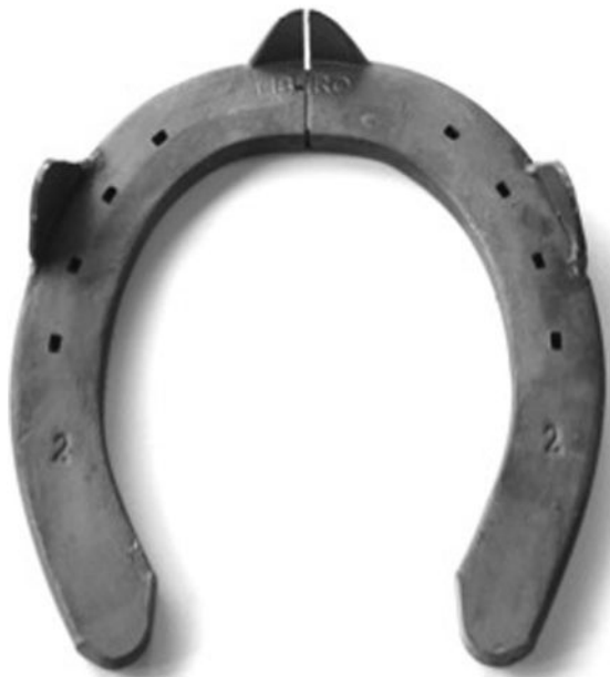
Fig. 1. The split-toe shoe is based on a conventional shoe with a toe clip and two side-clips between the second and third nail hole. The shoe is provided with a partially split toe that is sawn through after being nailed on the hoof, resulting in two halves moving independently.
